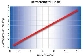
Refractometer Reading at 10% = 6.8 <sup>o</sup>Brix Refractometer Factor = 1.47
