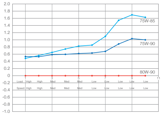
Synthetic 75W-90 and 75W-85 % Torque efficiency versus 80W-90 at a static operating temperature of 79.4°C/176°F
